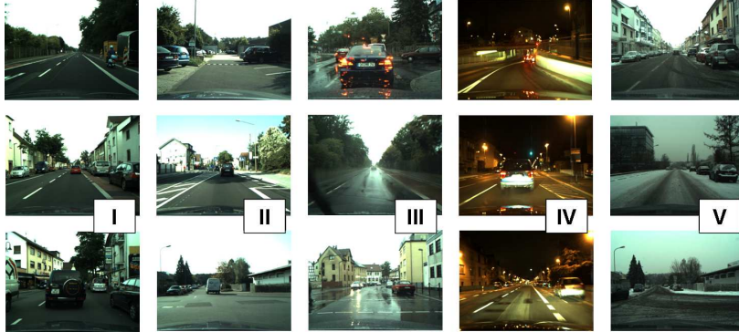
Figure 1: Selected example images from streams I-V. All videos were taken in RGB color using a MatrixVision mvBlueFox camera at a resolution of 800x600. Used frame rates were 10Hz except for video II where a setting of 20Hz was used. Aperture was always set to 4.0 except for video IV where we used a value of 2.4. A self-implemented exposure control was used on both cameras, manipulating the gain and exposure settings of each camera.
